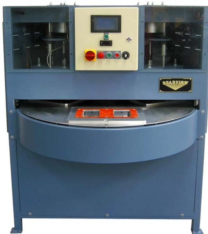
**Starview's new PHS3-1418 Three station semi-automatic Rotary Clamshell and Blister Sealing Machine.**
